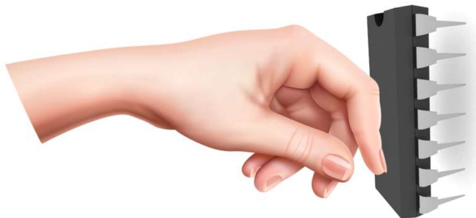
Fig. 1.22:Temperature test of IC using finger touch
