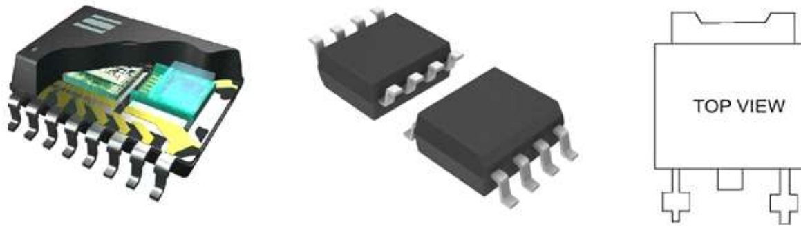
Fig.5.6: Small Outline Integrated Circuits (SOIL)
